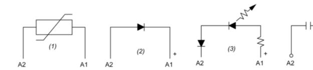
(1): MOV Suppressor(2): Protection Diode(3): LED Indicator(4): RC Suppressor
